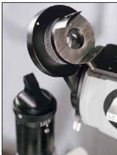
Figure 2: Remove material as needed to accommodate the flash unit.
